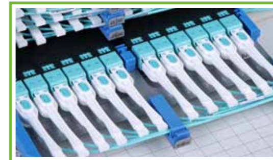
1 Duplex LC Connector Duplex LC to improve the installation density
